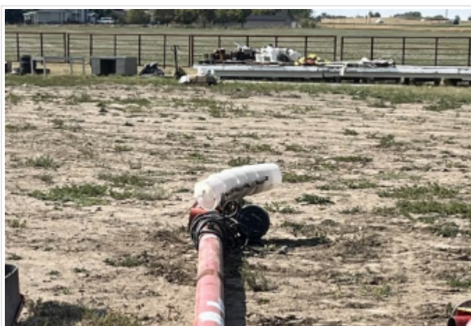
#4770E 25' x 6" pencil auger with electric motor
